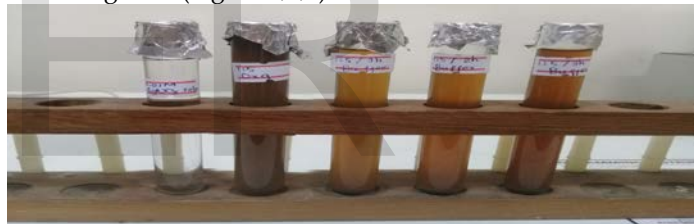
(a) (b) (c) (d) (e) Figure 1 Colour Changes of AgNPs (reducing agent: AgNO 3 ), (1:3) (a) AgNO 3 Solution (0.001M) (b) Fabrication of silver (after 10min) (c) Fabrication of silver (after 1h) (d) Fabrication of silver (after 2h) (e) Fabrication of silver (after 3h)
