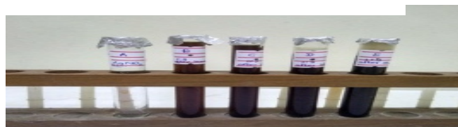
(a) (b) (c) (d) (e) Figure 2 Colour Changes of AgNPs (reducing agent: AgNO 3 ), (1:5) (a) AgNO 3 Solution (0.001M) (b) Fabrication of silver (after 10min) (c) Fabrication of silver (after 1h) (d) Fabrication of silver (after 2h) (e) Fabrication of silver (after 3h)
